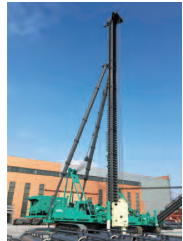
Pile driving rig
