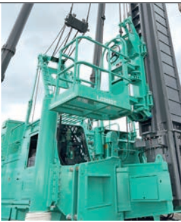
▲LG200T lifting work surface
