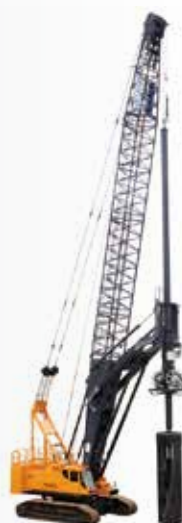
Earth Drilling Rig
