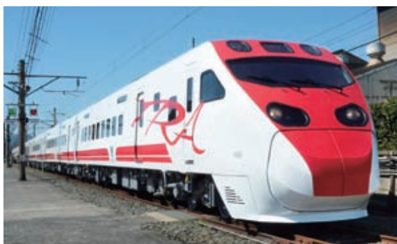
EMU with Tilting System for Taiwan
